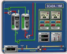
Supervisory Control And Data Acquisition System (SCADA)
